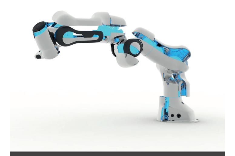
Joint torque controlled with a sense of touch
